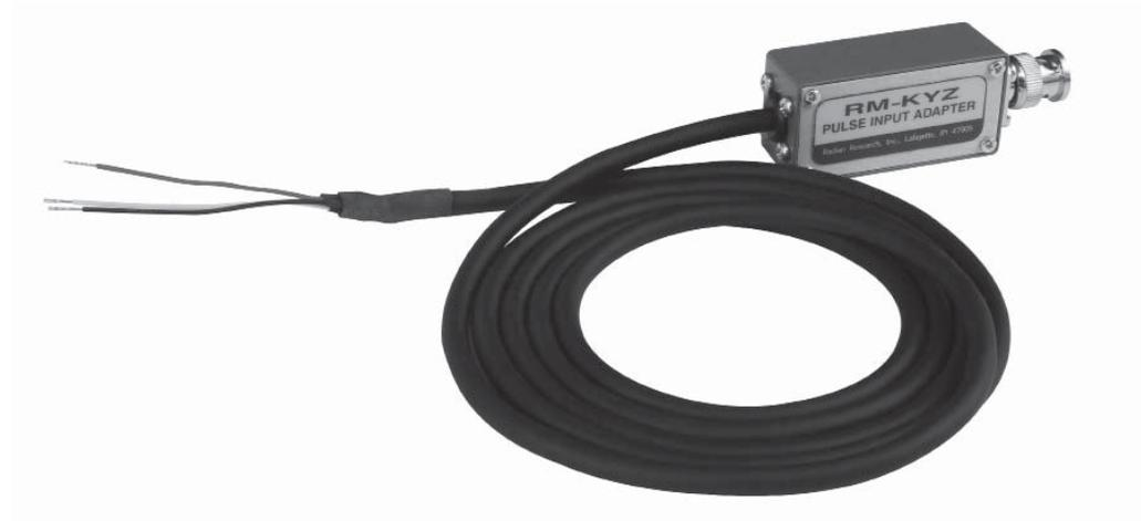
The **RR-KYZ Pulse Input Adapter** is used to sense the KYZ output pulses of an induction type or solid state meters. The pulses received from the meter's KYZ output are conditioned and fed into the PICKUP port of the RM-111 Automated Comparator. With the RR-KYZ and the RM-111 the testing of KYZ equipped meters is done automatically.
