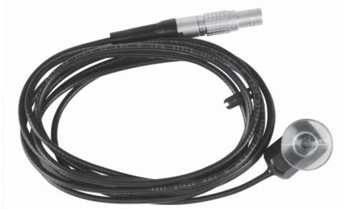
The **RM-OA Optical Adapter** is used with solid state meters whose infrared calibration pulses are emitted from the optical communications port. The RM-OA magnetically couples to the communications port of solid state meters. The suction cup of the RM-1H is attached to the clear polycarbonate cover of the RM-OA. The RM-OA incorporates a rare earth permanent magnet for exceptional holding power over the life of the product.
